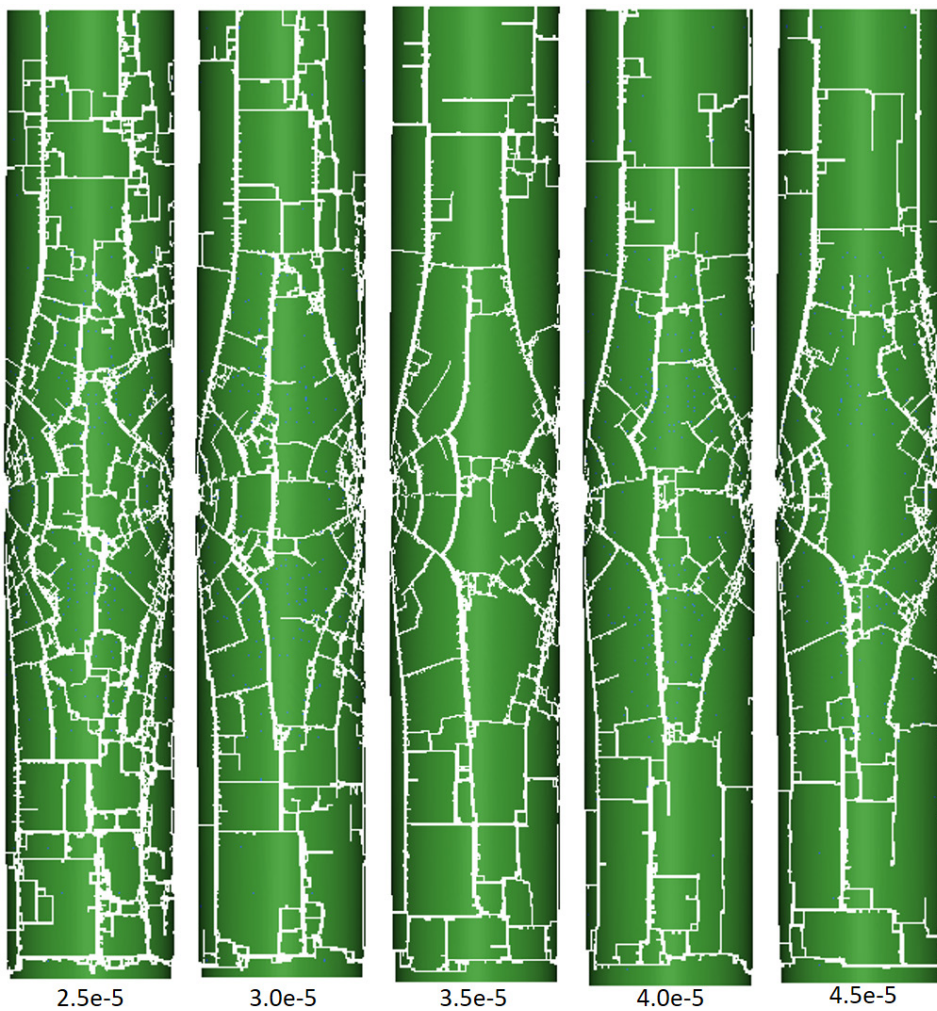
Figure 1-9: Near field search for max. principal strain with 0.5e^{-6} interval [3].
